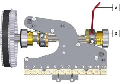
10. Turn the output shaft of the motor gearbox until the system is completely opened. (manually or by control box). In this example this end position corresponds with direction I.
